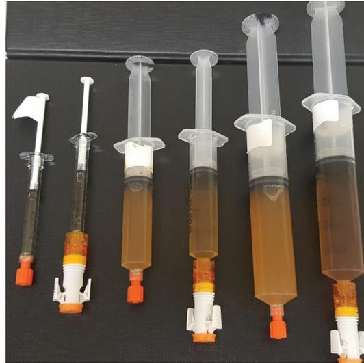
Figure 4. 50mL physical dye intrusion test (lower) versus the 50mL positive control (upper). Presence of MB dye in the positive control syringe only.
