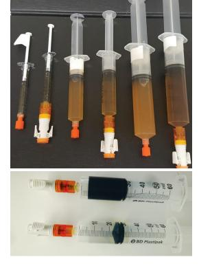
Figure 4. 50mL physical dye intrusion test (lower) versus the 50mL positive control (upper). Presence of MB dye in the positive control syringe only.
