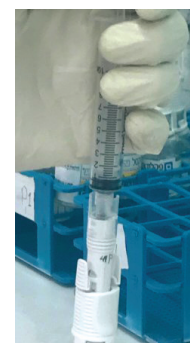
Figure 5: Injection of solvent to the vial using a Syringe Adaptor to Vial Adaptor system
