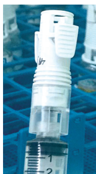
Figure 2: Assembly of a Syringe Adaptor to syringe
